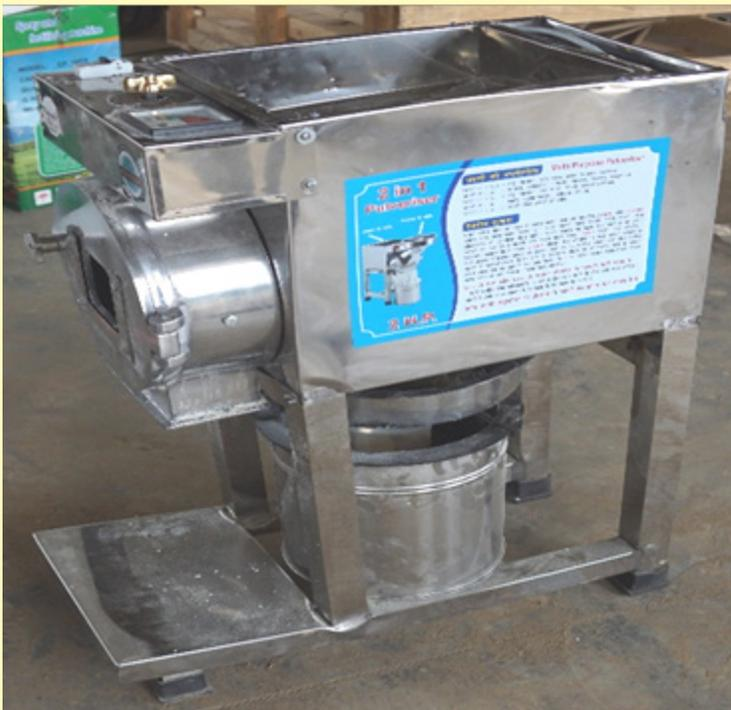
*Dry Grinding Machine (DGM)*
