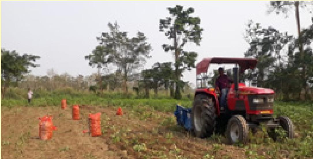
*Harvesting of Potato using Potato Harvester (tractor drawn)*
